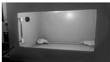
Fig. 1. The utilized unit for combined exposing of test animals to the whole body hyperthermia and injection of developed nano-fluids.
